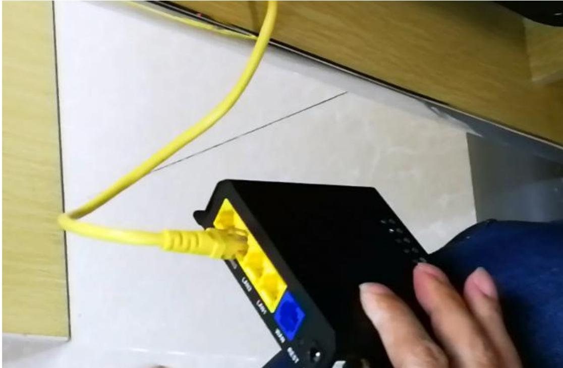
2,Keep pressing RESET button with sharp tool, then connect DC power adapter. Please wait for 15 seconds to boot up router. (Attention: Keep pressing RESET , and do not release it during 15 secs )
